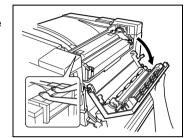
3 While moving the green lever on the inside of the upper right-side door in the direction of the arrow, carefully pull out the paper.
